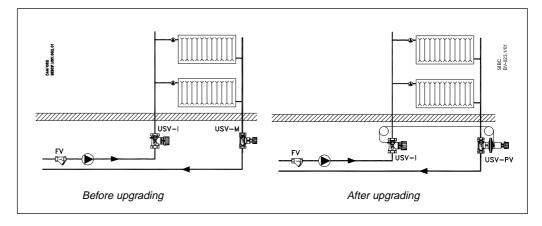
Upgradable USV valves are to be used for manual as well as automatic balancing of heating systems. If system has to be fitted with differential pressure controller, USV can be upgraded with PV controller.
