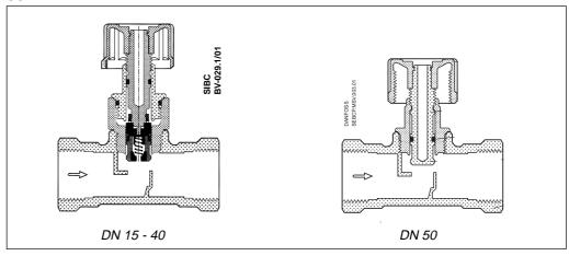
USV-M can be upgraded to USV-PV automatic balancing valve. The system does not need to be depressurized during the upgrade.
