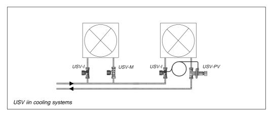
Upgradable USV control valves are to be used for manual or automatic hydronic balancing of cooling devices i.e. as fan coils or chilled ceilings.
