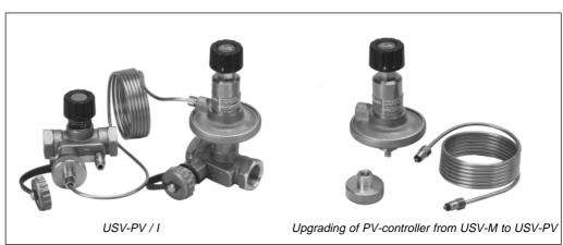
USV-PV (blue knob) is designed to maintain a constant set differential pressure across a riser. Eventual operating noise caused by high differential pressure induced by changes in the system can be avoided by upgrading the manual valve to the differential pressure controller.
