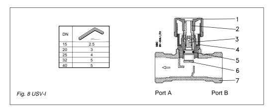
USV-I incorporates a double cone (3,6) able to give maximum stroke limitation, thus achieving flow limitation. It also incorporates shut off function. ASV-I is equipped with the nipples for the flow measurement and a connection for the USV-P/PV impulse tube.
