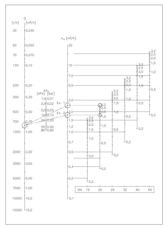
A straight line connecting the bars of flow, differential pressure and  $k_{\nu}$  value shows the relationship between these three variables.
