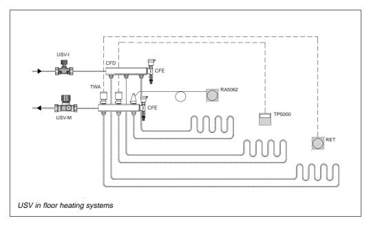
Upgradable control valves are to be used for manual balancing of a floor system manifold.
